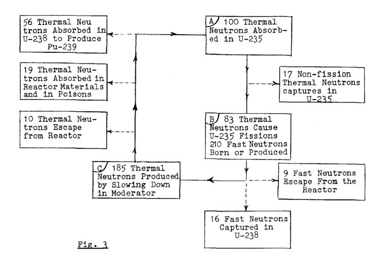
Finally 56 neutrons suffer radiative capture in U-238, so that the total neutron radiative capture losses in the fuel is 56 + 17.
